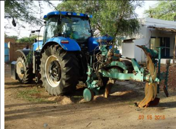
Picture 1 : Vallerani tractor of AGED for the mechanical work of the half-moons
